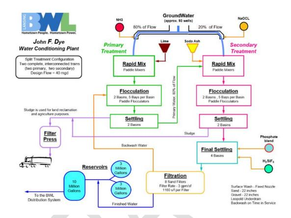
**Figure 9 - Dye WCP Treatment Process**
