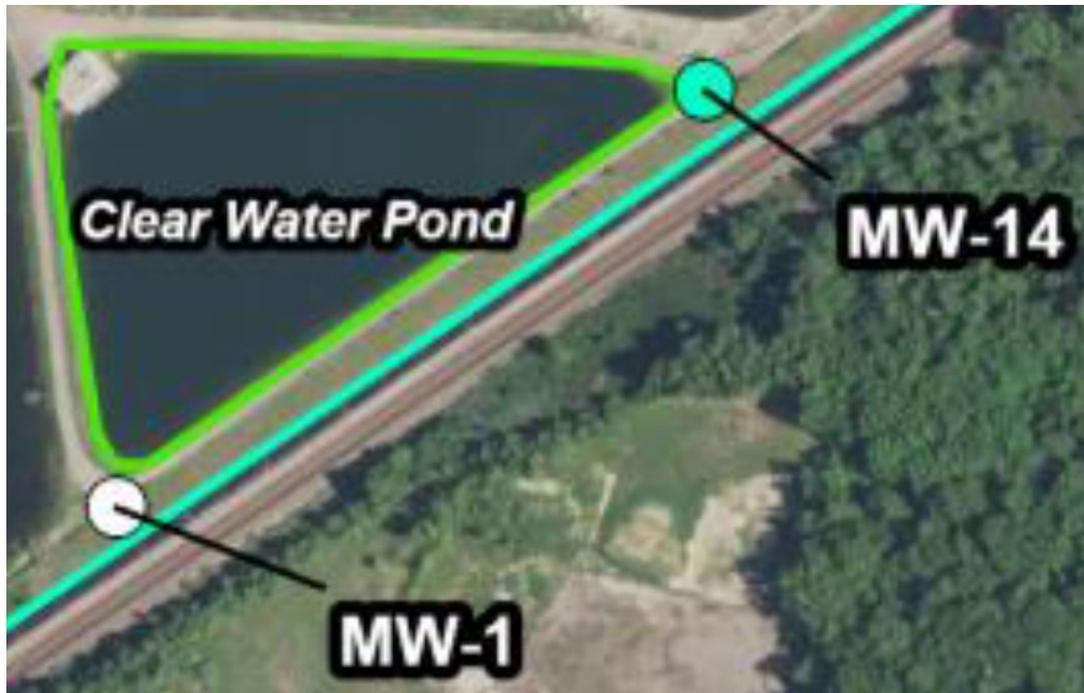
Figure 6. Monitoring Well Locations – Clear Water Pond
