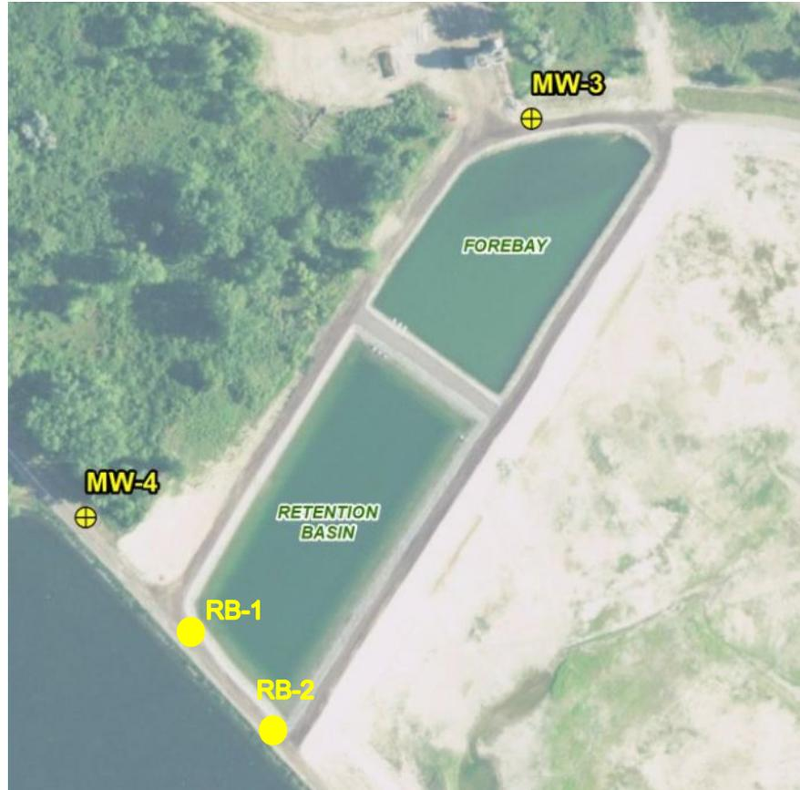
Figure 4. Monitoring Well Locations - Forebay and Retention Basin
