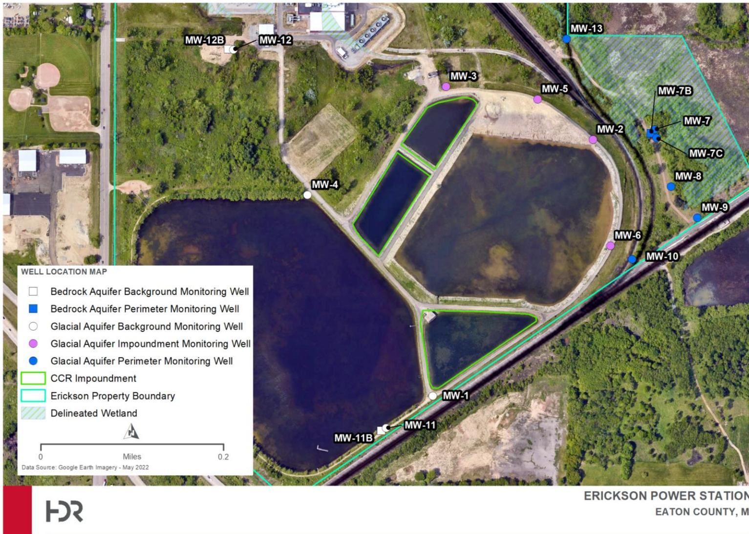
Figure 3. Erickson Station CCR Units and On-Site Monitoring Wells.
