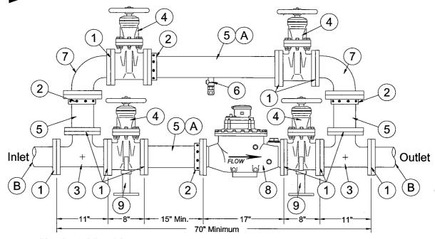
Must be 12" (Min.) from back wall with 3' working clearance in front of meter setting.
