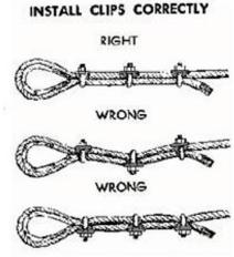
Correct way to apply U-bolts to form an eye in wire rope.
