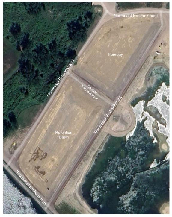
Figure 3. Forebay and Retention Basin Embankment Terminology
